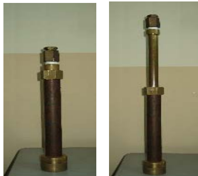
Figure 2. Before and after Photos; operation of Water Curtain Nozzles
