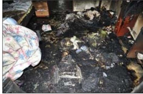
Fig.3. Burned feature of Point of origin.
