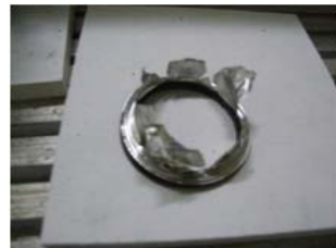
Figure 4. Pressure vessel tester and orifices and rupture of the disc
