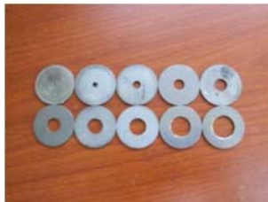
Figure 4. Pressure vessel tester and orifices and rupture of the disc
