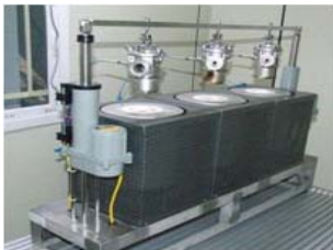
Figure 4. Pressure vessel tester and orifices and rupture of the disc
