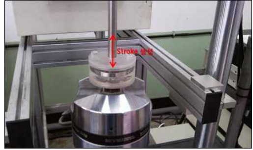
Figure. 2 Photograph of practical viscoelastic damper experiment
