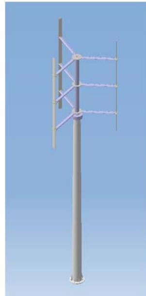
Fig. 3 Geometry configuration of 6 kW VAWT full model
