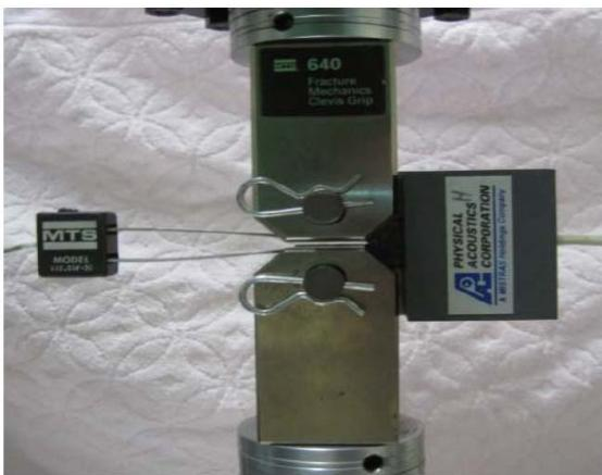
Fig. 2 Installation of AE sensor
