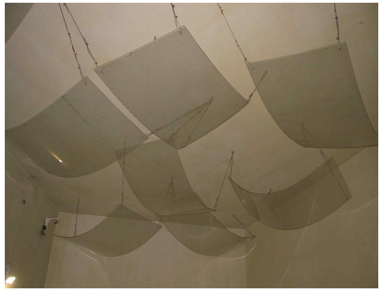
Fig. 1 Suspended diffuser in reverberation chamber
