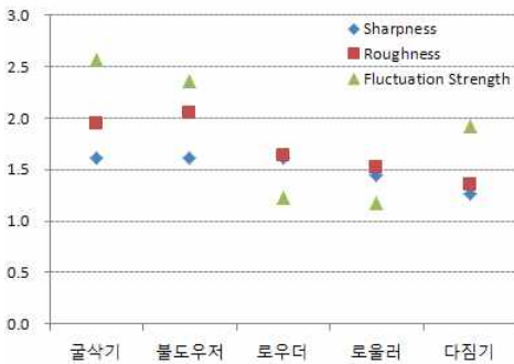
Figure 3. Sharpness, Roughness, Fluctuation strength of construction machinery noise
