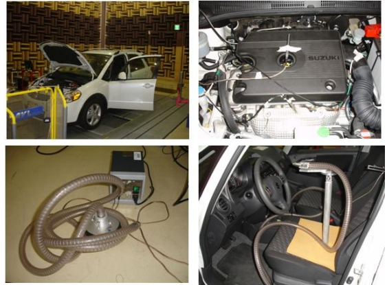
Fig. 1 Vehicle Noise Reduction Test Set-up
