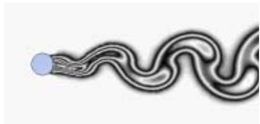
Fig. 1 Flow-field due to wind vortex around the tower.
