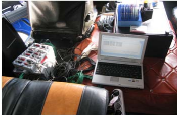
Figure 2 DAQ system for vehicle road driving test
