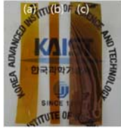
Figure 2 Transparent actuator: (a) Graphene electrode, (b) after electroless plating of Pt, (c) after sputtering of Au.
