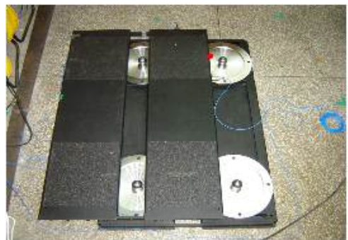
Figure 8. CFPBS seismic isolation system
