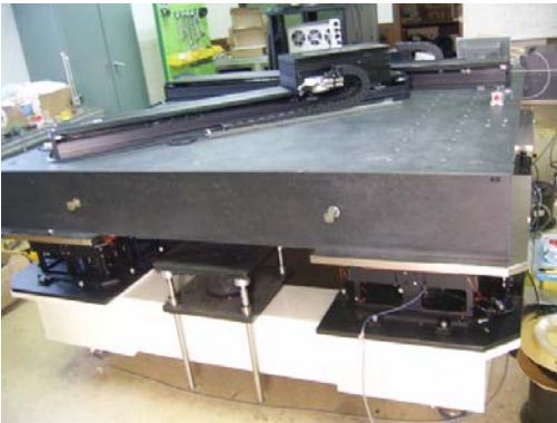
Fig. 2 An isolator combined with EM & MR in the test
