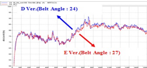
Fig. 5 FFT Analysis of changing Belt Angle
