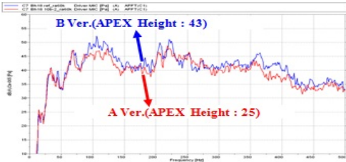
Fig. 3 FFT Analysis of changing APEX Height
