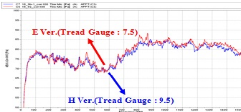
Fig. 4 FFT Analysis of changing Tread Gauge
