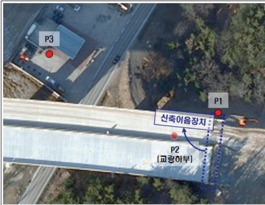
Figure 3. Position of noise source and receivers
