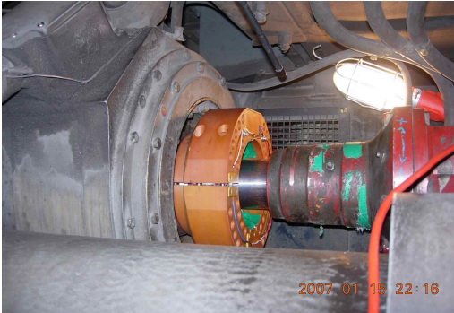
Fig. 2 Traction force measurement system of HSR-350x
