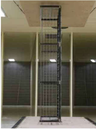
Figure 5 Catwalk models in wind tunnels
