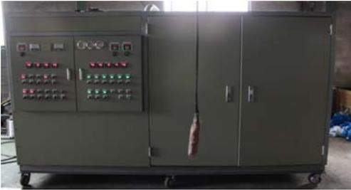
Fig. 1. Pyrolysis equipment for organic radwaste solution
