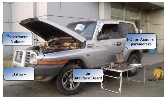
[그림 8] Setting for Experiment of Starting Engine
