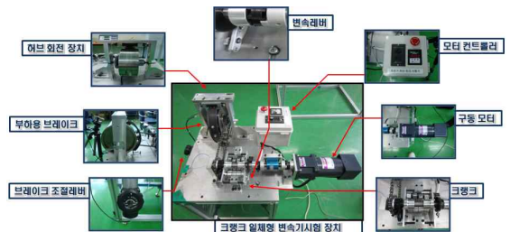
Figure 2 Test bench for measuring the transmission combined built-in crank performance
