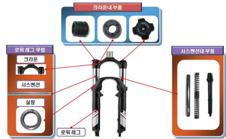
Figure 8 Structure of bicycle front suspension
