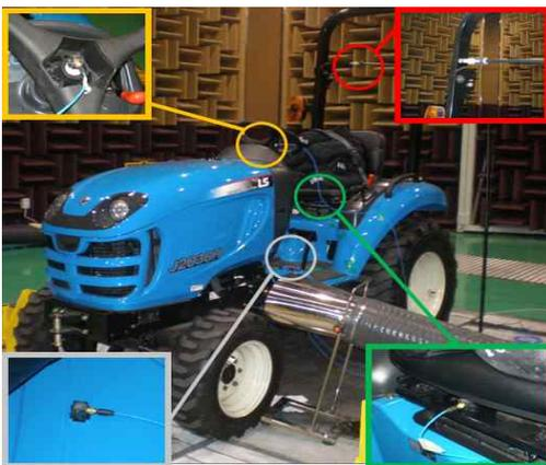
Figure. 1 Test Tractor and Measuring Position
