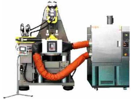
Figure. 2 3-Axial Elastomer Testing System
