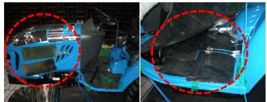
Figure. 3 Anti-Vibration Pad Applied to Top and both sides of Hood and Floor
