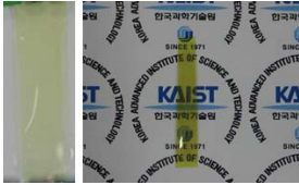
Figure 2 Transparent SPUI actuator with graphene electrodes.
