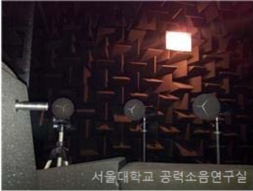
Figure 3 Measurement setup in anechoic chamber
