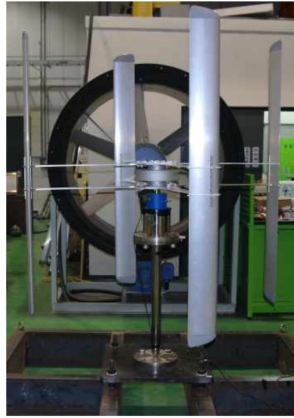
Fig. 3 Wind turbine installation on the tunnel Ground Base
