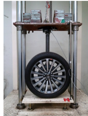
Fig. 3 Experimental apparatus for vertical tire stiffness test
