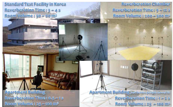
Figure 1. Various floor impact sound measurement conditions
