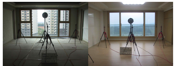
(a) with paper (b) without paper Figure 2. Measurement conditions of reverberation time in apartment buildings before moved in
