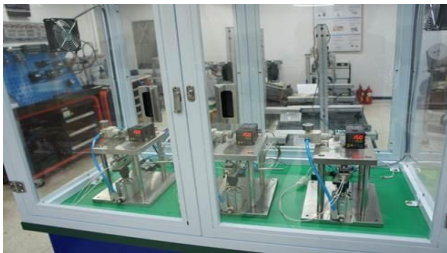
Fig. 5 Safety chamber for reliability test
