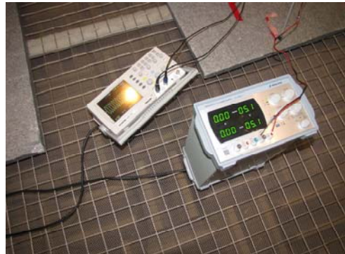
Fig. 3 SMD microphone sensitivity test in balanced signal mode vs. various power supply voltage.
