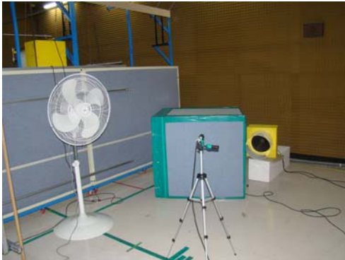
Fig. 4 Measurement set-up for testing sensitivity to wind interference
