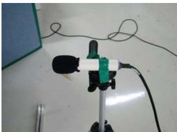
Fig. 4 Measurement set-up for testing sensitivity to wind interference
