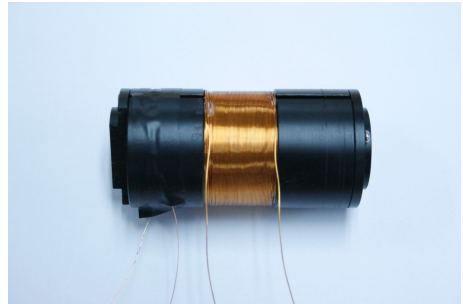
Fig. 1 Semi-active tuned mass damper
