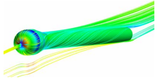
Fig. 6 Stream line plot at M= 0.85 and \alpha = 6^\circ .
