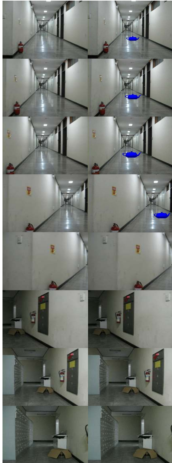
Figure 5. Example of the experiment. (left) The sequences of original video and (right) is the video after 3D object insertion. The figure shows frame 1 st , 162 nd , 347 th , 515 th , 560 th , 624 th , 688 th , and 767 th frame where we can assume that the camera go straight, turn left and go forward again.
