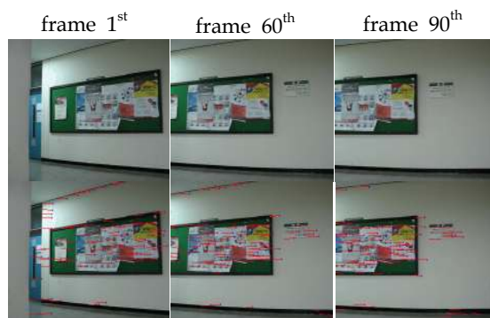
Figure 1. (Top) Example of frames in video. (Bottom) Using the red lines which show optical flow, we can assume that the camera turned to the right side.
