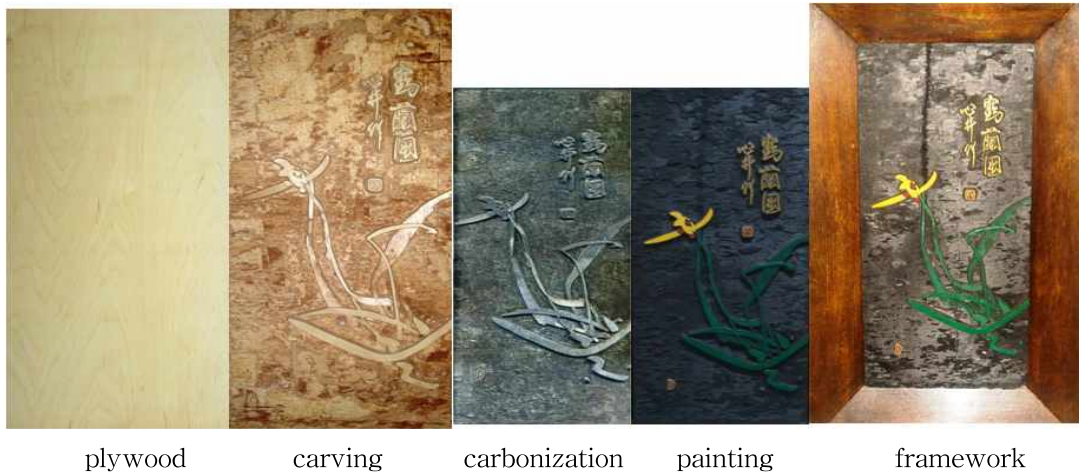
Fig. 3. Manufacturing process of calligraphy-carving carbonized artwork from plywood.
