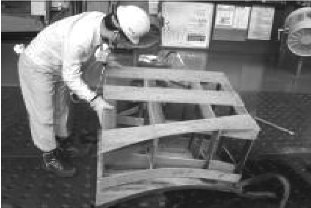
Fig. 2 Box Template for shell plate forming
