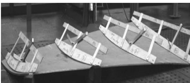
Fig. 1 Template for shell plate forming
