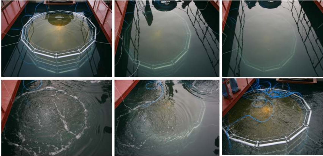
Fig. 3. Model submersible fish cage system during lowering(upper) and raising(below) by air control system.
