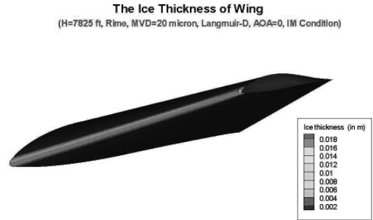
Fig 6 Ice thickness (H=7825 ft, Rime, IM)
