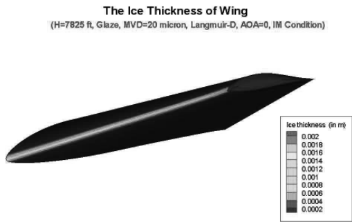
Fig 5 Ice thickness (H=7825 ft, Glaze, IM)
