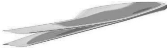
Fig.9 Initial and converged wing shape ( M=0.75 , AoA=0 deg, Re=3 \times 10^6 )
