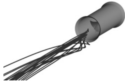
Fig. 9 Streamlines near the outlet of jet fan
