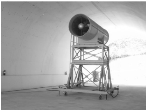
Fig. 2 Photograph of jet fan
