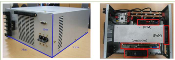
(b) inverter stack
