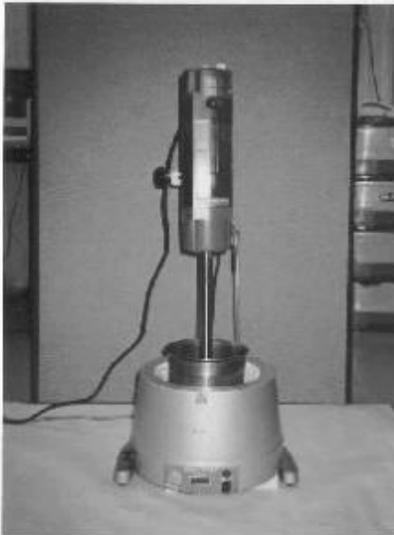
Fig. 7. Homogenizer.
