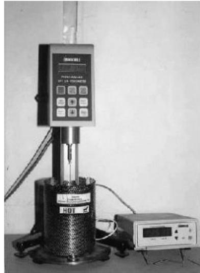
Fig. 8. Brook field viscometer.
