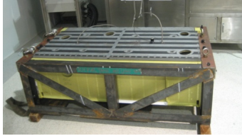
Fig. 11 Pressure test after slosh & vibration test
