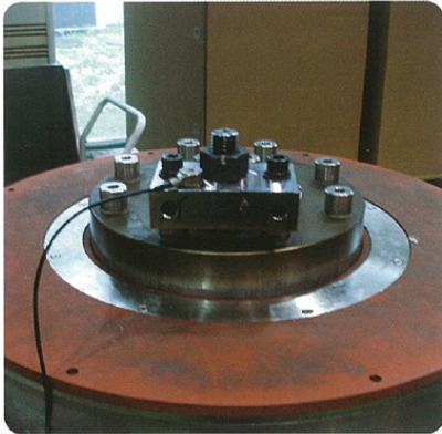
Fig. 9 After KS R9186 test of M20
