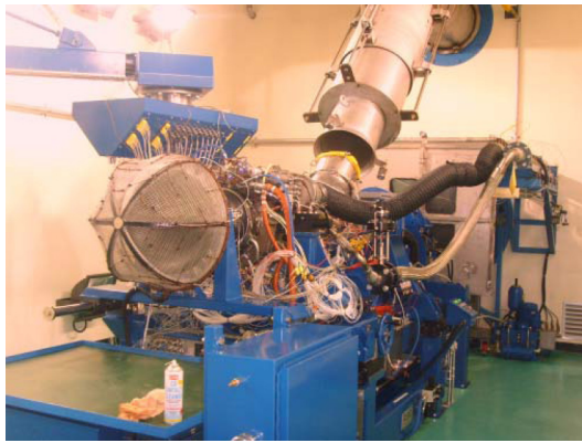
(b) T700/701K Engine Test Cell
