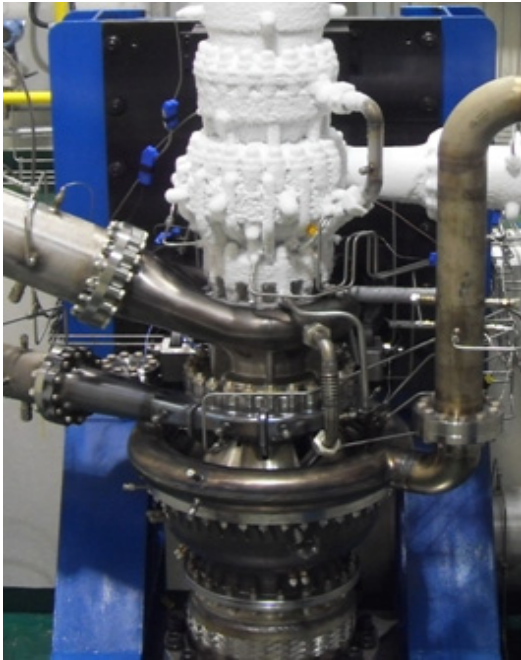
Fig. 3 Configuration of turbopump assembly test
