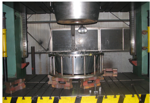
Fig. 4 Forming process of outer jacket
