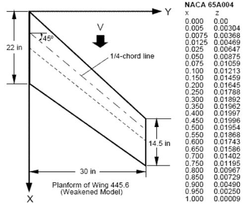
Fig. 1 Geometry of AGARD 445.6 test case [6]
