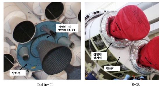
Fig. 2 Heat Shield in Delta-II and H-2B
