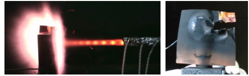
Fig. 4 Damage of the brass plate by the flame of TM-OS-02
