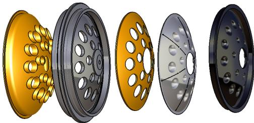
Fig. 1 CAD Drawings of Pulse Separation Device
